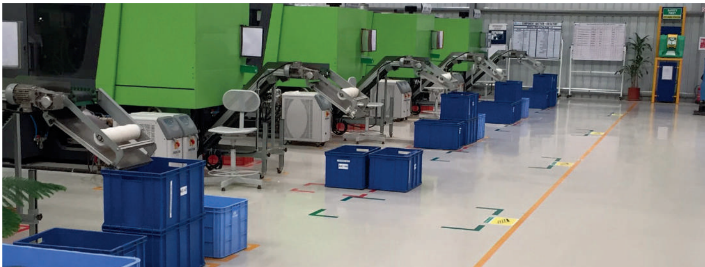
Complete organisation of the site in compliance with the 5S method - Location of cases and pallets at the output of the machine
